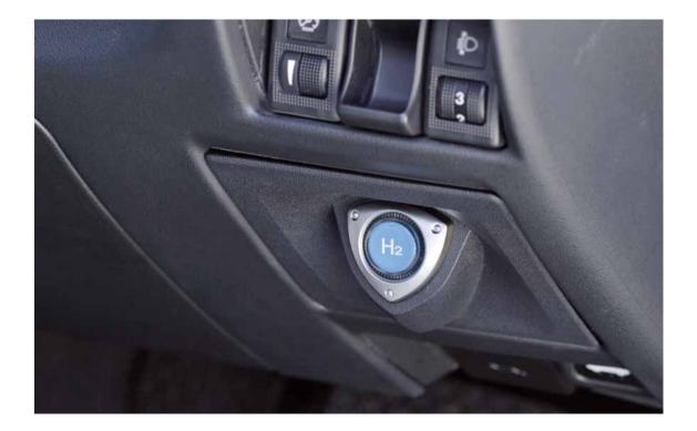
Switching from hydrogen gas to petrol can be done using the switch next to the driver's seat. The car must be stationary to switch from petrol to hydrogen. In addition, when the hydrogen tank is empty, the RX-8 Hydrogen RE switches automatically to petrol power.
