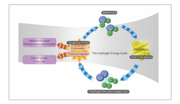
Hydrogen combustion follows the simplest of chemical formula: two H2 molecules combine with an O2 molecule to form two H2O molecules in vapour form, while at the same time releasing a very large quantity of energy. This reaction produces extremely few NOx nitrogen oxides and gives off no CO<sub>2</sub> (a greenhouse gas) whatsoever.
