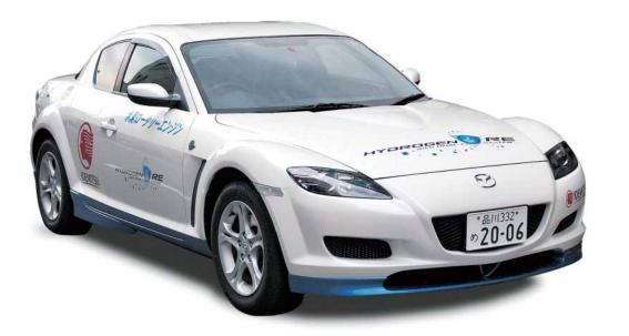
A world first: the Mazda RX-8 Hydrogen RE is the first hydrogen internal combustion passenger car supplied for lease. Idemitsu Kosan Co. Ltd. in Tokyo and Iwatani International Corporation in Osaka were the first two companies to take this pioneering step, following Hiroshima City and Prefecture.
